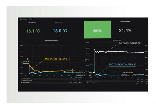
Thanks to its interfaces, the technician can monitor the temperature in each tank, mass percentage of salt in the brine or seawater, as well as the freezing point value of the liquid.
